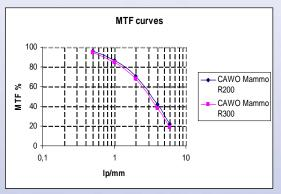
The MTF curve results from measurements which indicate a degree of the "intrinsic sharpness"of the film-screen system as perceived on the image. The total image quality depends on other factors besides the "intrinsic sharpness". The main factors are: graininess, noise, film, contrast, optical density and aesthetic aspects like image tint, etc.
