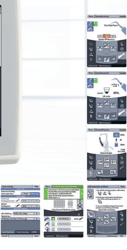
The well-designed graphical user interface offers ease-of-use and a multitude of user-specific settings and parameters. All instrument and unit functions can be controlled either from the GUI touch screen or from the unit foot control. While the GUI information screen displays the functions that are activated, the GUI control screen displays the functions operated from the foot control and/or the touch screen.
